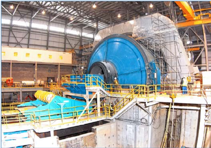
40-foot SAG mill with wrap around motor
