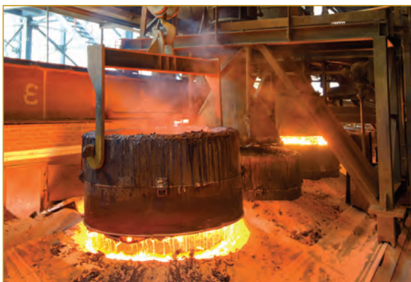
Ferromolybdenum production at the Langeloth Metallurgical Facility
