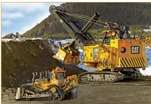
Electric-powered shovel at Mt. Milligan, British Columbia
