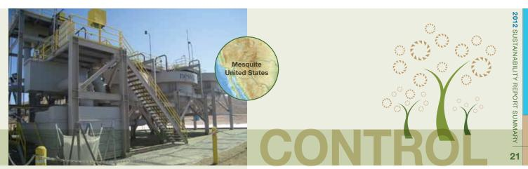
Carbon-in-columns tanks at Mesquite, where cyanide solution is prepared and applied in full compliance with ICMC.
