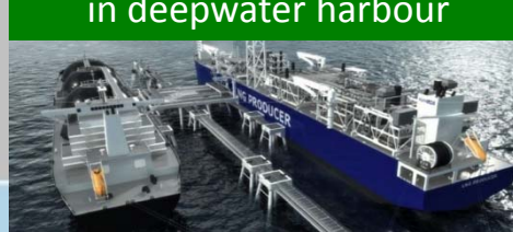
Floating LNG vessel moored in deepwater harbour
