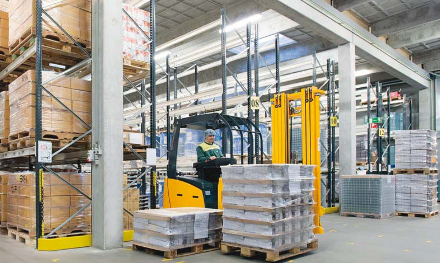
Efficient narrow-aisle forklift: The battery-powered, tri-lateral EFX 410–413 stacker can be operated freely in wide aisles and even unload lorries if necessary.
