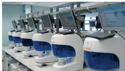
Above: Dental milling machines at central manufacturing facility in Stonehouse
